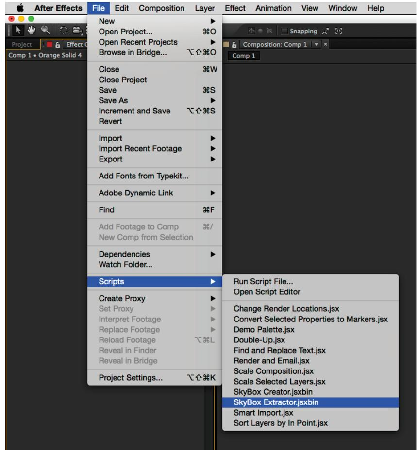
**SkyBox Extractor** removes the Equirectangular distortion in 360 footage and then extracts 6 camera views. Extractor then positions them in a cube formation in After Effects in a “SkyBox Edit” comp pictured below.
